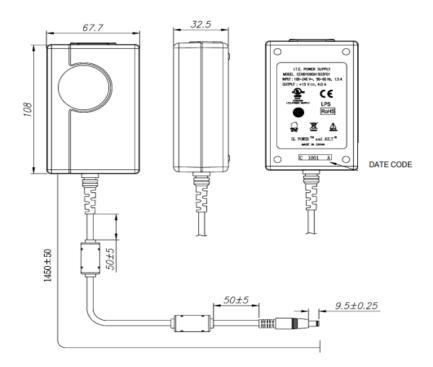
Dimensions are in mm (Cable length is 1500mm on12V thru 24V models)
