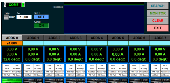
Figure 3: GUI, 24 V TF Series power supply connected to ADDS 0 at COM7 in remote mode (orange)
