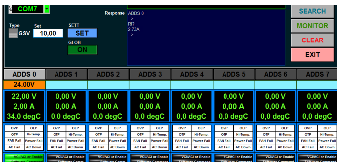
Figure 6: GUI, response to executed command "RI?"
