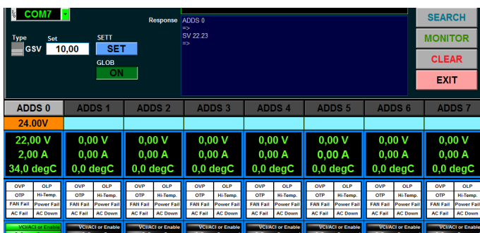
Figure 4: GUI, response to executed command "SV 22.23"
